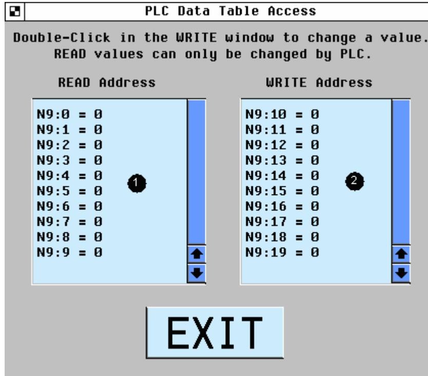
① This scrolling window displays the PLC addresses that are being read from the PLC and the associated values. These values can only be changed from the PLC.
